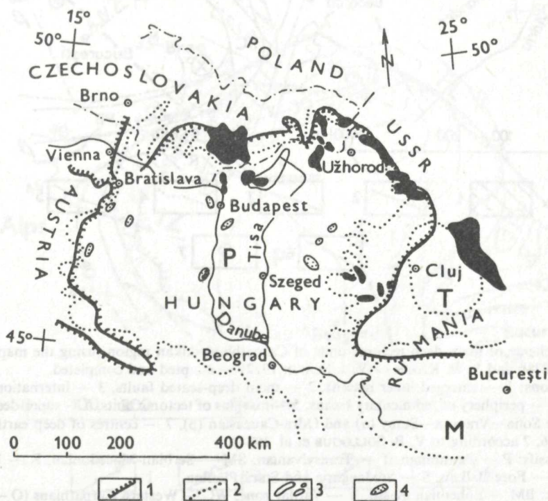
Fig. 29 Extent of Carpathian-Balkan region disturbed by positive gravity in relation to Inner-Carpathian Neogene basins.
